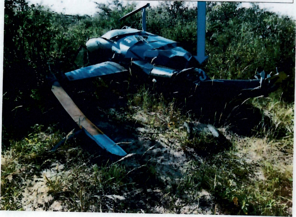
Closer view of the same picture above, showing extensive damage by the root of tail boom.
